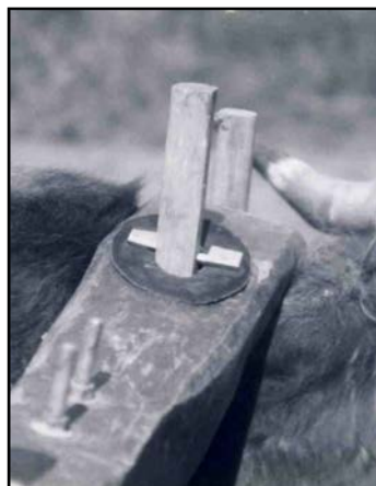
A leather washer will prevent key from damaging the top of the yoke.
