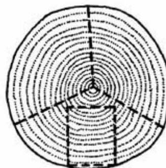
Diagram 2. Endgrain view showing how yoke can be cut from one third of log.
