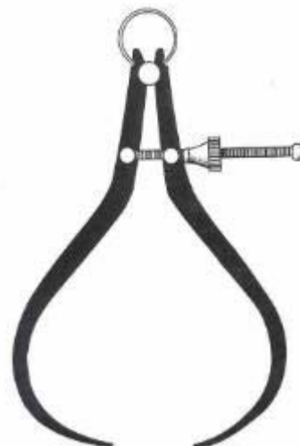
This is an Outside Caliper, used to take dimensions of the diameter of round surfaces.
