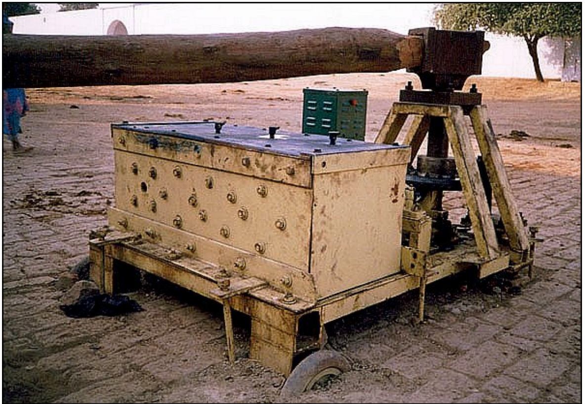
Bullock (ox) powered generator which can give 2 bulb electricity to 50 houses in India's villages
