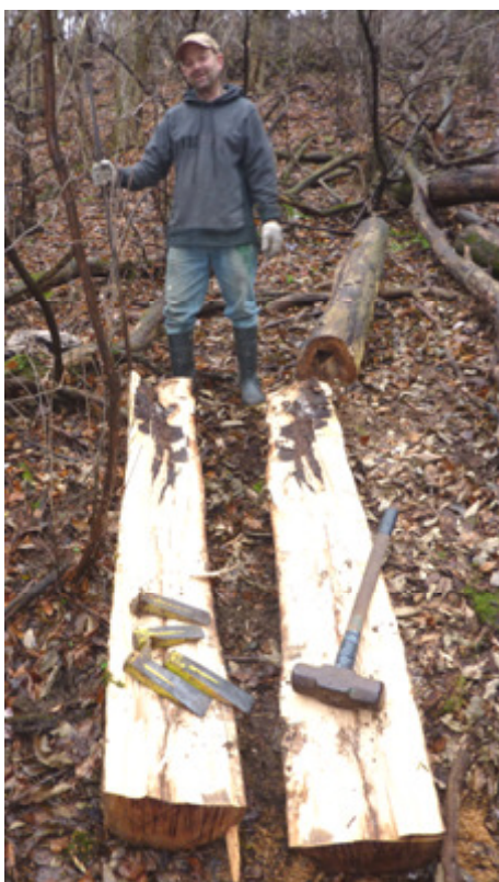
Caitanya, has just split this locust post in half....this section yielded four posts.
