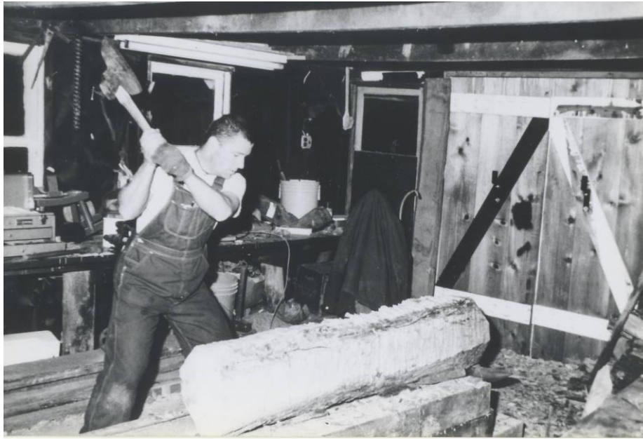
Picture 2. Here I'm using a broad ax to hew the log.
